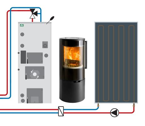
With various smart EnergyFlex accessories, you can connect and control external heat sources such as water-jacketed stoves, solar collectors and wood, pellet, oil or gas boilers.
