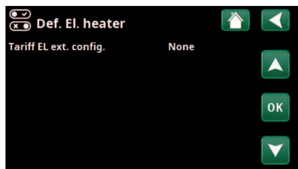
Menu: "Installer/Define/Immersion heater".
