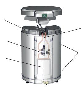
Connection via top mounting (accessory) is fully concealed. The pipe is run through ducts in the cover and the connection is fully concealed by the front panel
