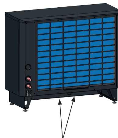
Condensate tray and condensation water drain.
